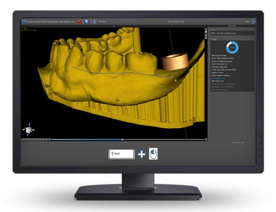
The hole in the brown software guide tube represents the exact location and size of the hole that will exist in the printed surgical guide.
