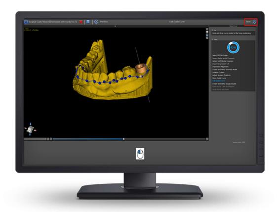
Hold the left mouse button to Grab and drag any of the nodes that appear along the surgical guide curve to fine tune the curve positioning and to straighten any crossed segments.
