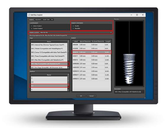
Select "Mandible" as the Implant Orientation. Select "Blue Sky Bio" from the "Implant System" drop down. Select the BIO | Max implant type, 4.3mm implant platform, and select the 10mm implant.
