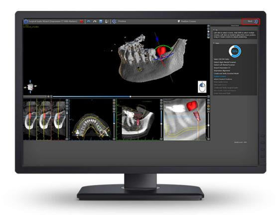
Now, in any view, use the left mouse button to move and rotate just the implant placement without affecting the placement of the tooth. The keyboard arrows can also be used to nudge the implant placement in small increments.
